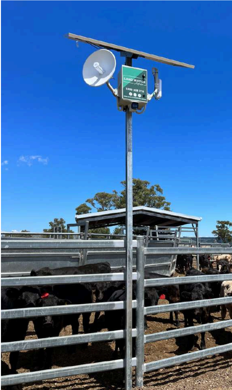
4 kilometer Land Watch Link with repeater, camera and wifi
